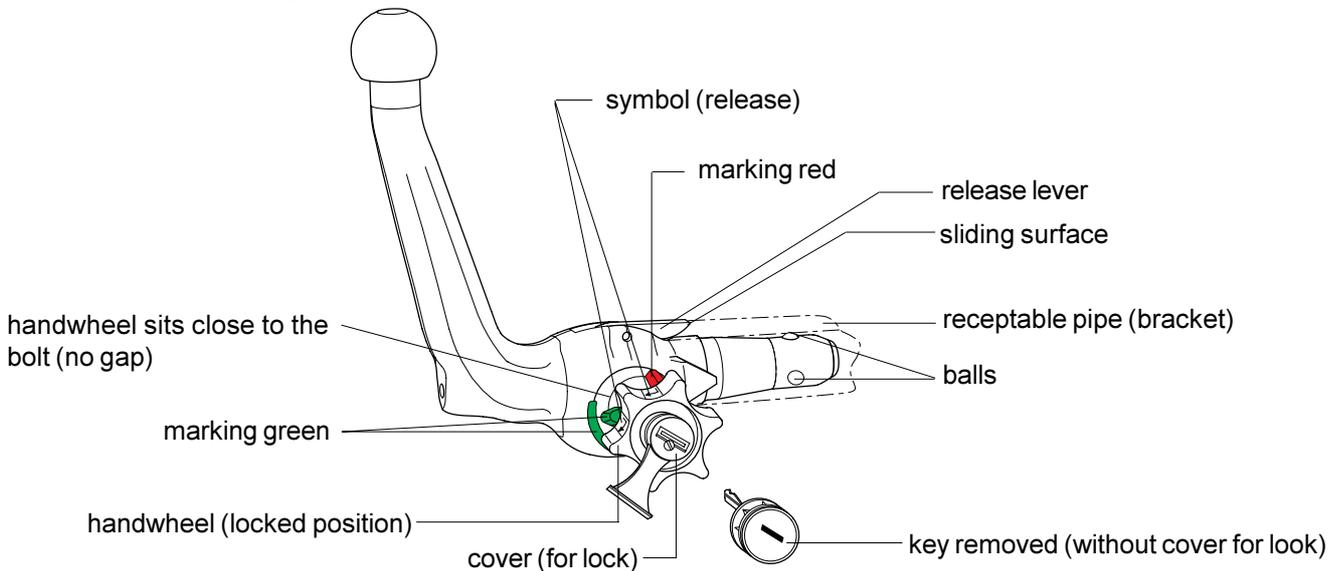
**Unlocked position (coupling hitch unmounted)**
