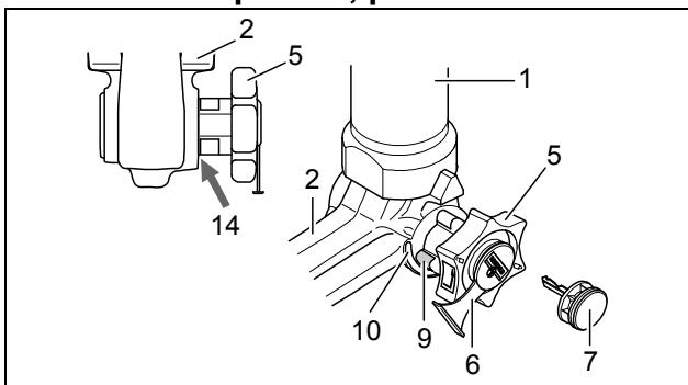
**Odjištěná poloha, odpojeno**
