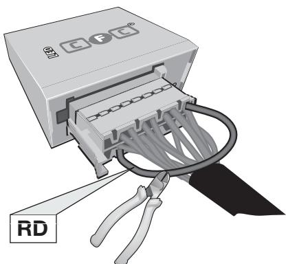
Pin 11 and Pin 2 disconnected
